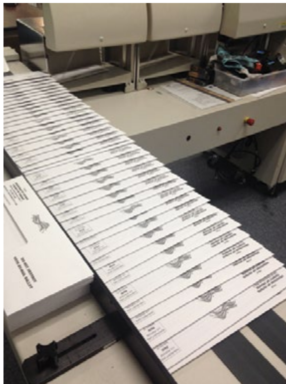
Orange County's in-house mail processing equipment automatically labels envelopes and inserts ballots.
