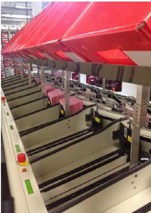
Sacramento County's vote-by-mail processing equipment sorts ballot envelopes from the June 2014 primary election.
